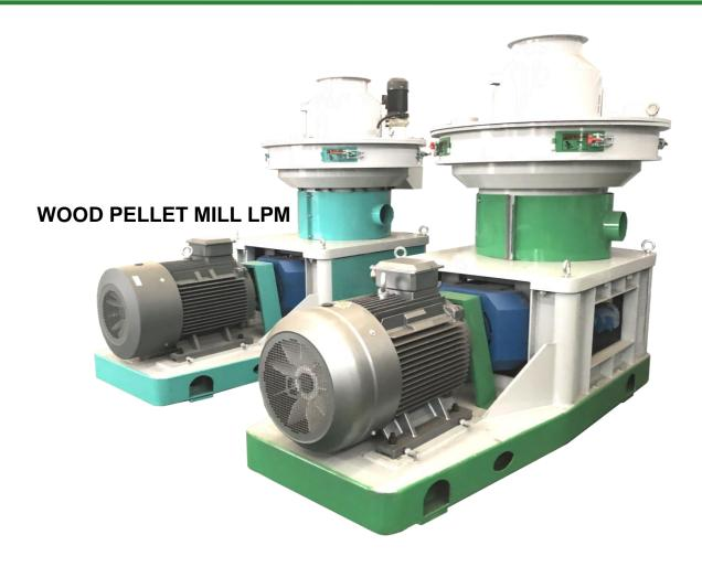
The LPM series pellet mill is suitable to make pellets from crushed and dried powder, such as rice husks, sawdust, cotton stalks, cottonseed skins, rank grass, and other crops straw, plant waste. Our equipments are widely used in power plant, wood processing plant and biomass fuels plant.
