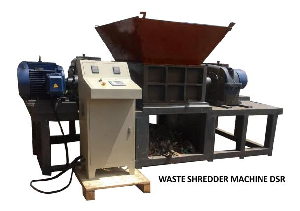
The waste shredder machine is a very useful equipment for processing large volume and heavy duty of waste, such as reams of paper, paper materials, bumpers, tires, refrigerators and the shredding of different materials like scrap iron, aluminum, copper, plastic as well as municipal solid waste and industrial waste.
